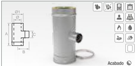
Colector vertical entronque Ø80 (Inox 316-Interior / Inox 304-Exterior)
